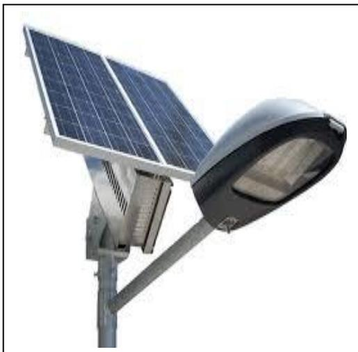
Solar Street Lights operates from Dusk to Dawn automatically switches ON after the sunset and switches OFF after sunrise. These street lights operate in standalone mode. The solar street light should be installed in a shadow free area or place where direct sunlight is available throughout the day. Street lighting system consists of SPV Module, Charge Controller Unit, Battery, Luminary, Interconnecting Cables and Pole.
